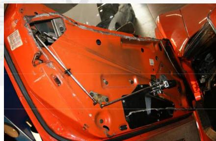
Remove the kick plate to gain access to the factory bolts. There are 4 in each hinge.
