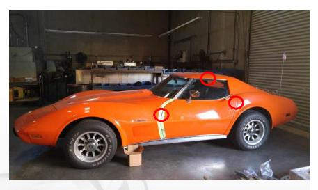
Remove the door panel. This will give you access to the bolts securing the door to the factory hinge.
