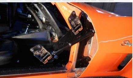
Tighten the bolts on the new VDI Hinge.
