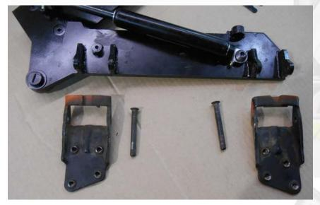
Separate the factory hinges into two halves by removing the original hinge pin (using a hammer and a punch) You will use the door half, set aside the body half.
