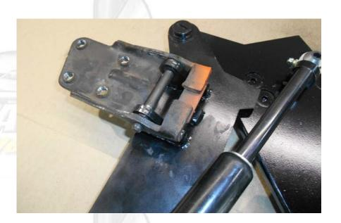
Install the factory hinge onto the new VDI Hinge using the original hinge pins and a hammer.
